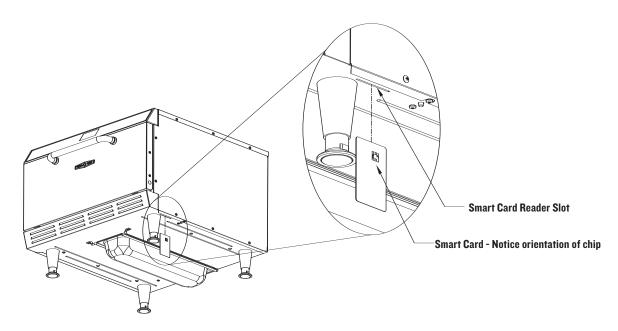
FIGURE 19: Inserting Smart Card into Reader
